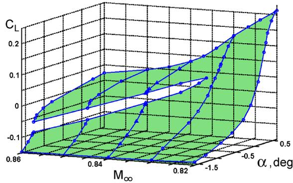
Figure 2: Lift coefficient as a function of the angle of attack and free-stream Mach number for turbulent flow over J-78 airfoil. Computations using the  $k - \omega$  SST model on a mesh of 135,078 cells at  $Re = 5.7 \times 10^6$ .
