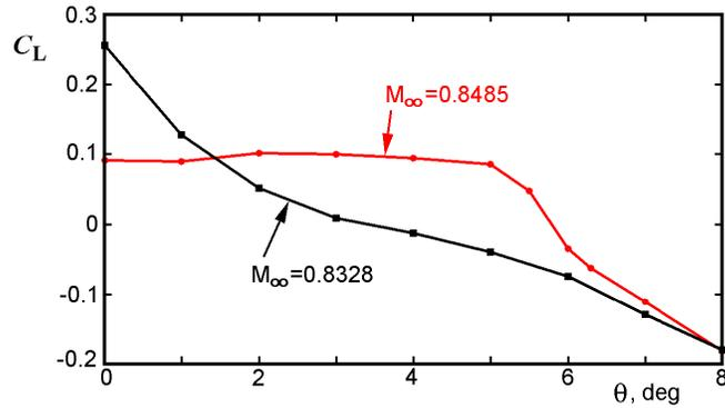
Figure 12: Lift coefficient versus the aileron deflection angle  $\theta$  for transonic flow over the airfoil (1) at  $\alpha = 0$ ,  $Re = 5.1 \times 10^6$ . Computations using the  $k - \omega$  SST turbulence model.
