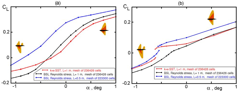
Figure 4: Lift coefficient as a function of the angle of attack for J-78 airfoil calculated at  $Re = 5.7 \times 10^6$ ,  $T_\infty = 220$  K using two turbulent models and two lengths  $L$  of the airfoil chord: (a)  $M_\infty = 0.82$  ( $U_\infty = 243.9$  m/s), (b)  $M_\infty = 0.84$  ( $U_\infty = 249.8$  m/s).
