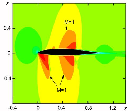
Figure 6: Mach number contours in transonic flow past the Boeing 737 Outboard airfoil at the Mach number  $M_\infty = 0.808$  ( $U_\infty = 256$  m/s), the angle of attack  $\alpha = -2$  deg, and  $Re = 5.7 \times 10^6$ .
