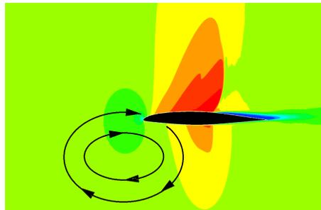
Figure 7: Sketch of an adverse free-stream vortex for the Boeing 737 Outboard airfoil in cruise conditions.
