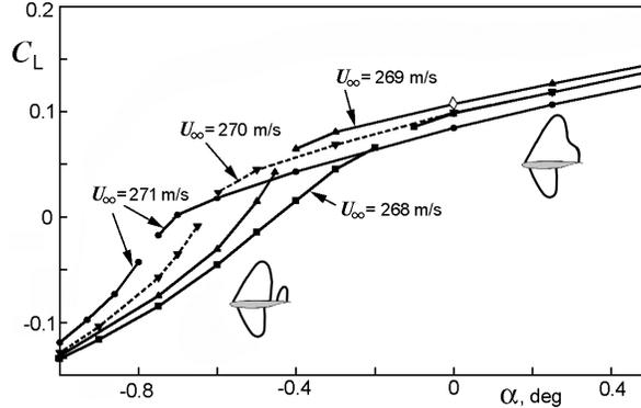
Figure 9: Lift coefficient as a function of the angle of attack  $\alpha$  for transonic flow past airfoil (1) at the aileron deflection angle  $\theta = 4$  deg,  $Re = 5.1 \times 10^6$ . Computations using the  $k - \omega$  SST turbulence model.
