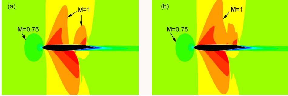
Figure 3: Mach number contours in turbulent flow over J-78 airfoil at  $M_\infty = 0.84$ ,  $Re = 5.7 \times 10^6$ ,  $L = 0.5$  m,  $k - \omega$  SST turbulence model: (a)  $\alpha = -0.64 - 0$  deg, (b)  $\alpha = -0.64 + 0$  deg.
