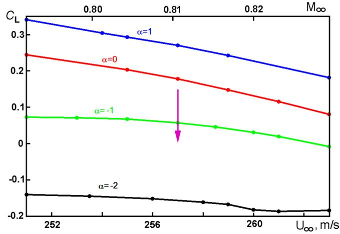
Figure 5: Lift coefficient versus the free-stream Mach number  $M_\infty$  and velocity  $U_\infty$  for the Boeing 737 Outboard airfoil. Calculations using the  $k - \omega$  SST turbulence model at  $Re = 5.7 \times 10^6$ ,  $T_\infty = 250$  K.
