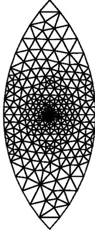
Figure 1: Sketch of the computational domain and mesh.
