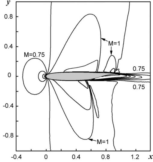
Figure 10: Mach number contours in transonic flow past airfoil (1) at  $\theta = 4$  deg,  $\alpha = -0.5$  deg,  $M_\infty = 0.8485$  ( $U_\infty = 269$  m/s),  $Re = 5.1 \times 10^6$ .
