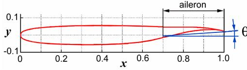
Figure 8: Sketch of the Whitcomb airfoil with an aileron deflected at an angle  $\theta$ .
