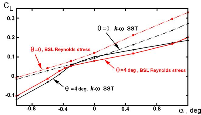
Figure 11: Lift coefficient versus angle of attack for transonic flow over the airfoil (1) at  $M_\infty = 0.8485$ ,  $Re = 5.1 \times 10^6$ .
