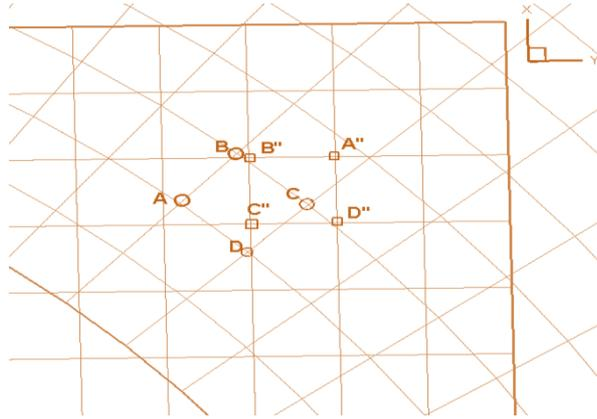
Fig.3 Interpolation on the overlapping grid points
