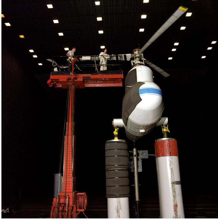
Figure 2: Experimental Set-up in the 80- by 120- ft Wind Tunnel (courtesy Wadcock and Yamauchi; Ref.6)
