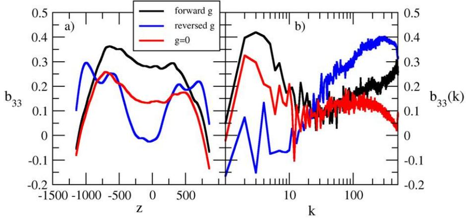
Figure 9: a) Vertical variation of  $b_{33}$  and b) scale dependence of the normal stresses anisotropy at the centerline, at the reference time.
