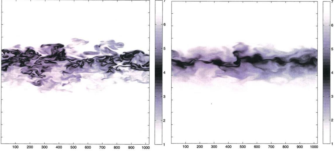
Figure 4: 2-D snapshot of the density field from the reversed gravity case at the a) reference time and b) late time.
