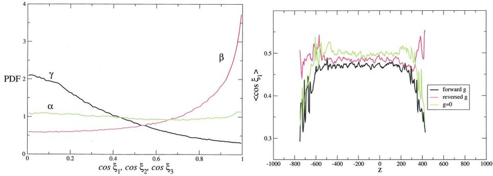
Figure 10: a) PDFs of the cosines of the angles,  $\xi_1$ ,  $\xi_2$ , and  $\xi_3$ , between the vorticity vector and the eigenvectors of the strain rate tensor for the reversed gravity case at the reference time. The eigenvectors correspond to the eigenvalues  $\alpha$ ,  $\beta$ , and  $\gamma$  denoted with the usual convention that  $\alpha > \beta > \gamma$ . b) Vertical variation of the average of  $\cos \xi_1$  for the three cases at the reference time.
