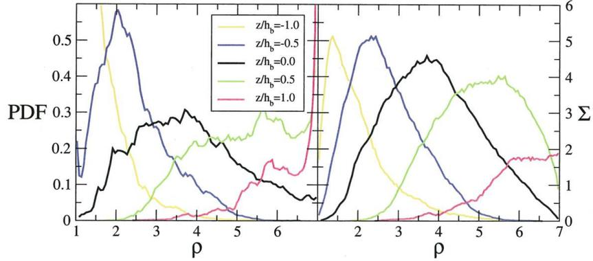
Figure 7: a) Density PDF and b) surface density function at several locations across the layer for the zero gravity case at late time.
