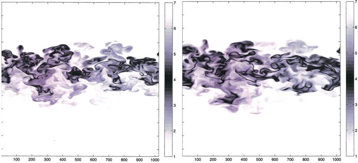
Figure 5: 2-D snapshot of the density field from the zero gravity case at the a) reference time and b) late time.
