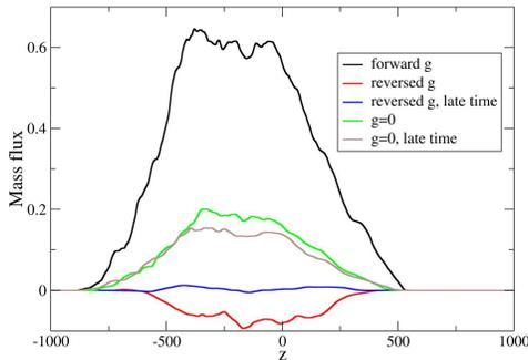
Figure 12: Mass flux variation across the layer for the three cases, at the reference and late times.
