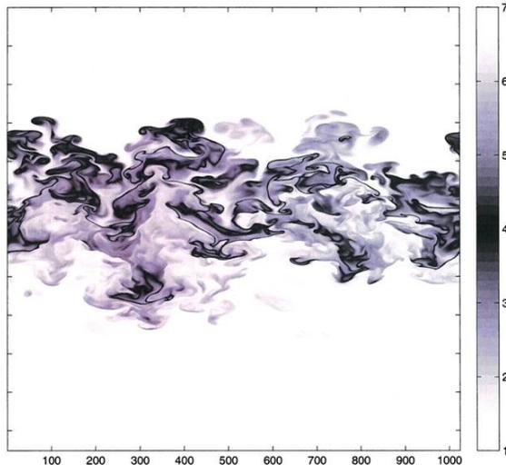
Figure 3: 2-D snapshot of the density field from the forward gravity case at the reference time
