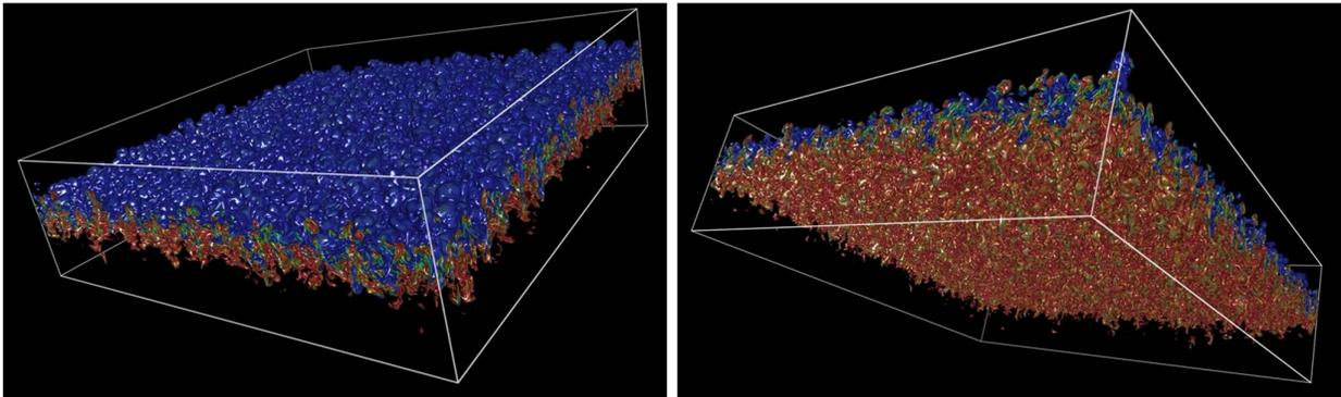
Figure 1: Three-dimensional visualization of the density field at early time, viewed from a) top and b) bottom, showing the asymmetry of the Rayleigh-Taylor mixing layer at  $A = 0.75$ , with the development of “bubbles” on the heavy fluid side and “spikes” on the light fluid side. From the  $4096^2 \times 4032$  simulation.
