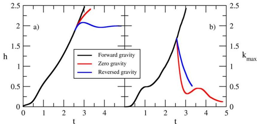
Figure 2: a) Layer width  $h$  and b) maximum turbulent kinetic energy across the mixing layer from an  $A = 0.75$  simulation. The main simulation (forward gravity) is branched into additional simulations with zero gravity and reversed gravity at time  $\approx 2.5$ .
