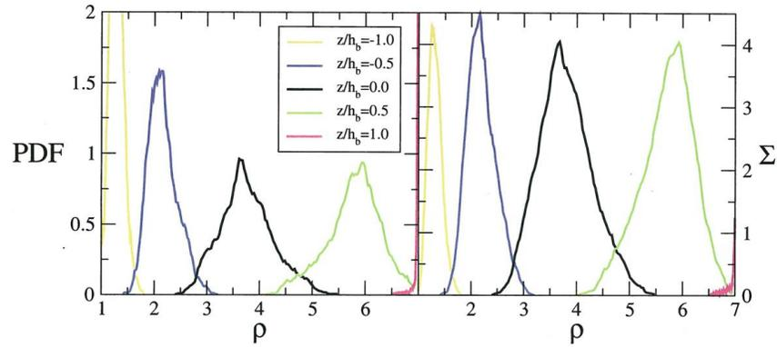
Figure 8: a) Density PDF and b) surface density function at several locations across the layer for the reversed gravity case at late time.
