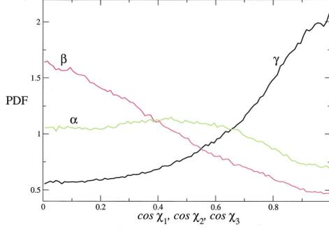
Figure 11: a) PDFs of the cosines of the angles,  $\chi_1$ ,  $\chi_2$ , and  $\chi_3$ , between the density gradient and the eigenvectors of the strain rate tensor for the reversed gravity case at the reference time. The eigenvectors correspond to the eigenvalues  $\alpha$ ,  $\beta$ , and  $\gamma$  denoted with the usual convention that  $\alpha > \beta > \gamma$ .
