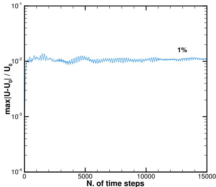
Figure 10: Velocity oscillations (spurious currents) for a translating sphere along the box diagonal, as a function of time.
