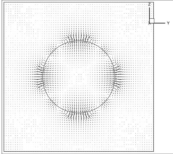
Figure 4: Spurious currents for the viscous 2D static droplet test with  $We_D = 1$ ,  $N = 64$ ,  $D = 0.5$ :  $C = 0.5$  isoline and fluid velocity vectors after 640 time steps.
