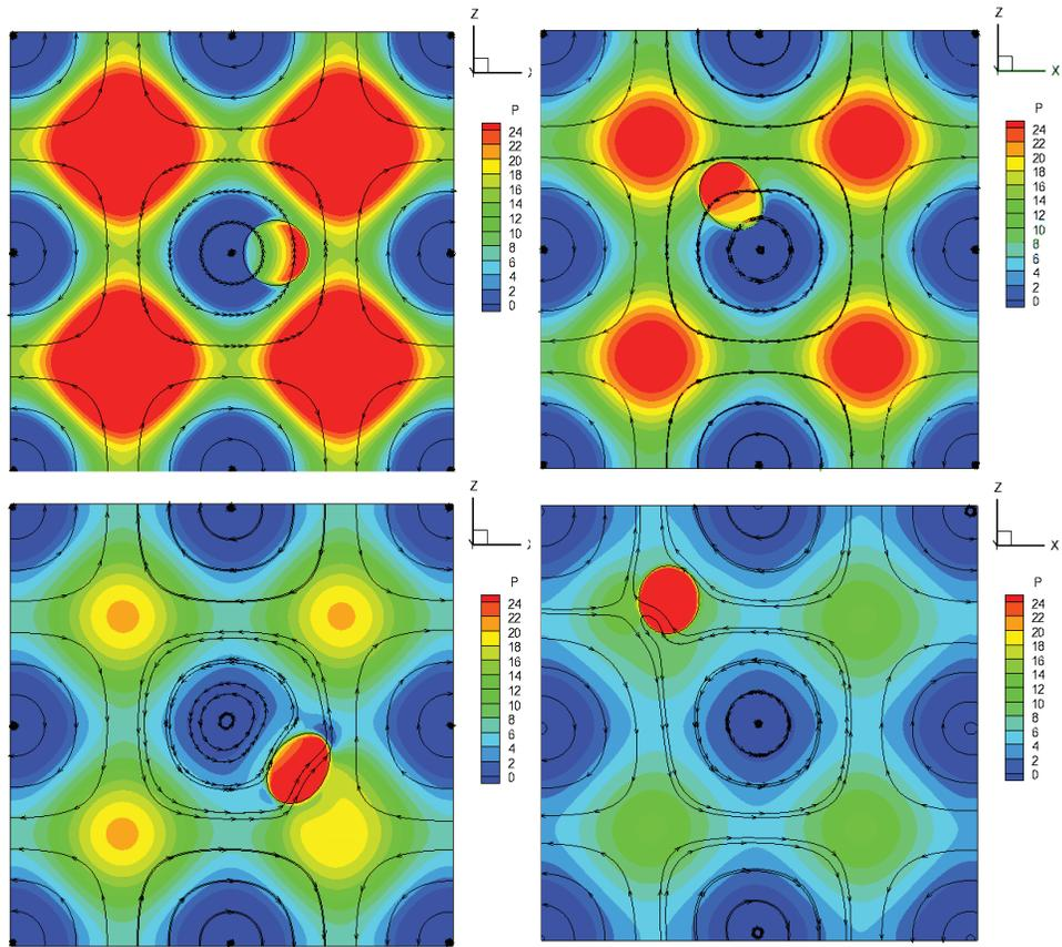
Figure 11: Instantaneous pressure contours, streamlines and droplet/fluid interface ( $C = 0.5$  isoline) for a droplet in the Taylor-Green vortex flow ( $We_D = 0.1$ ,  $N = 128$ ,  $D = 0.15$ ) at four different times.
