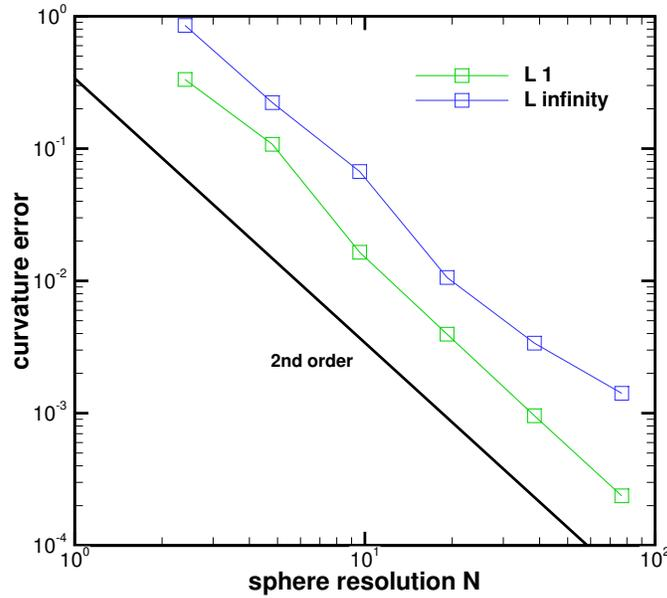
Figure 3:  $L_1$  and  $L_\infty$  curvature error norms averaged over 100 randomly placed spheres as a function of the number of grid points per sphere diameter.
