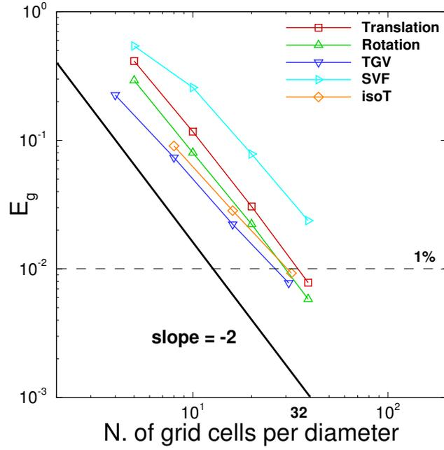
Figure 2: Geometrical error,  $E_g$ , of the advection and reconstruction algorithm for a sphere as a function of mesh resolution at CFL=0.1. Translation along the box diagonal, rotation and time-reversed single-vortex flow (SVF) with period  $T=2$  for a sphere of radius 0.15. Time-reversed Taylor-Green vortex flow (TGV) with period  $T=2$  for a sphere of radius 0.12. Time-reversed isotropic turbulence flow at  $Re_{\lambda_0} = 75$  (isoT) with period  $T=1$ .
