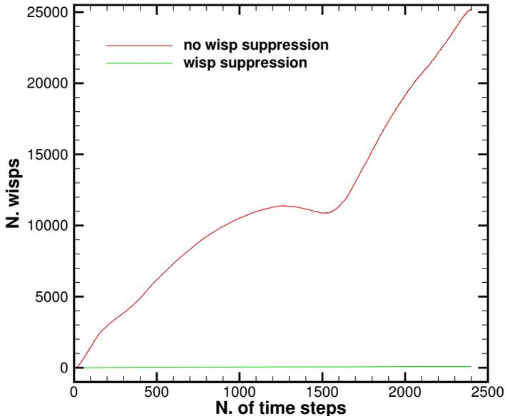
Figure 1: Total number of wisps vs number of time steps for a sphere of radius 0.15 advected in a time reversed single-vortex field [10] with period  $T=2$  using a mesh of  $128^3$  grid points.
