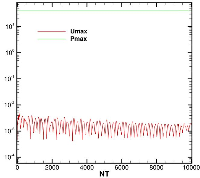
Figure 9: 3D viscous static droplet test at  $\sigma = 5$ ,  $N = 64$ ,  $D = 0.5$ . 8-fold symmetry enforced to the VoF function,  $C$ .
