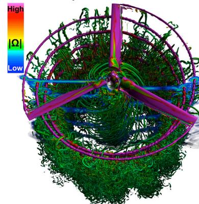
**Figure 4** OVERFLOW AMR hover simulation,  $M_{tip}=0.625$ ,  $Re=2.1$  million.
