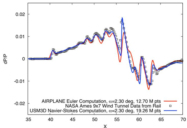
Figure 2. Lockheed Martin Configuration, Mach 1.6, height 80.8 cm.
