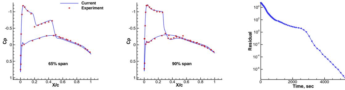
**Figure 1:**  $C_p$  distributions compared to experimental results of Schmitt and Charpin [10], and convergence plot for steady transonic flow ( $Ma=0.8395$ ,  $Re=11.72e6$ ,  $\alpha=3.06^\circ$ )
