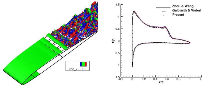
**Figure 2:** Q-criterion ( $Q=1$ ) coloured by streamwise vorticity and  $C_p$  plot overlaid by results from Zhou and Wang [11], and Galbraith and Visbal [12] for the SD7003 wing ( $Ma=0.2$ ,  $Re=60e3$ ,  $\alpha=4^\circ$ )
