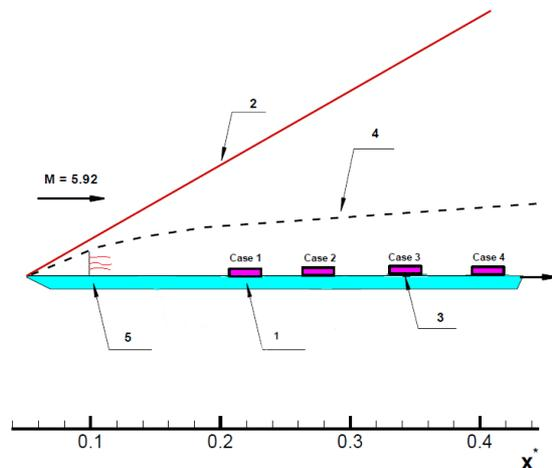
**Figure 1. A schematic of the problem: 1. Roughness 2. Bow Shock 3. Synchronization point 4. Boundary layer 5. Imposed disturbances**
