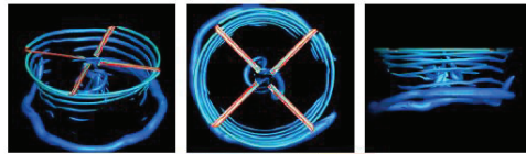
Figure 5. Vortex structure of the isolated PSP rotor
