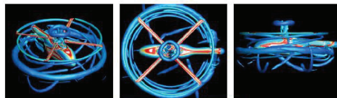
Figure 6. Vortex structure of the installed PSP rotor under free-air condition
