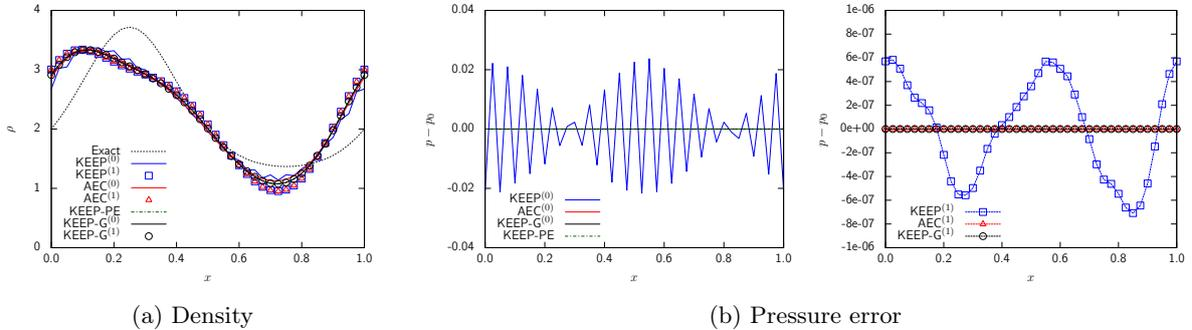
Figure 1: Instantaneous (a) density and (b) pressure-error distributions at  $t = 13$  for the 1D density wave advection.
