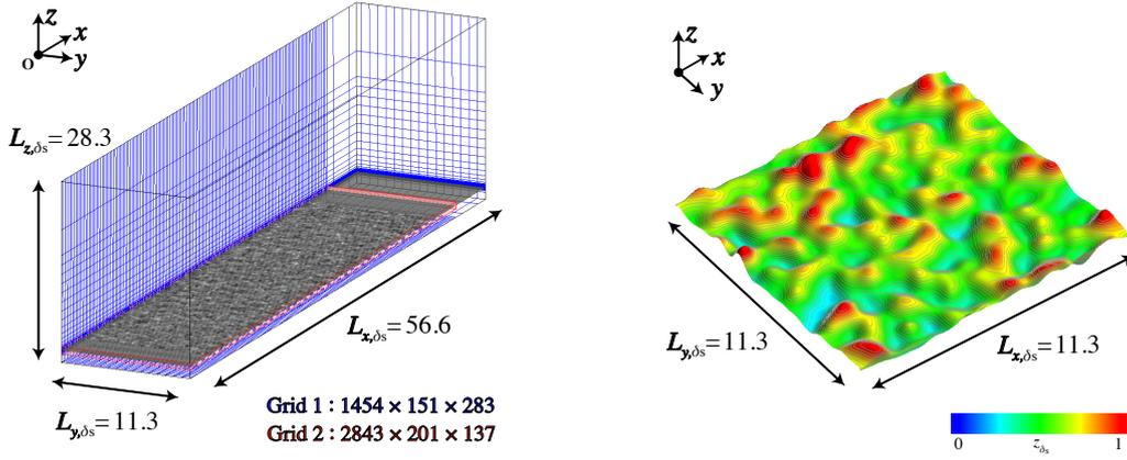
Figure 1: Computational grids and an example of gaussian roughness surface ( $\phi_{\delta_s} = 1.0$ ,  $\rho_{\delta_s} = 1.0$ )
