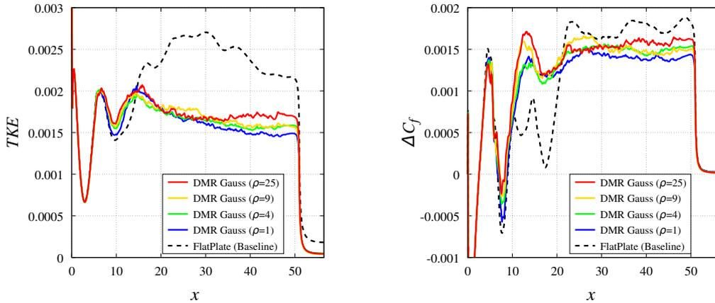
Figure 2: Friction drag coefficient ( $C_f$ ) and Turbulent kinetic energy ( $TKE$ ) integrated along the wall-normal direction at each position in the streamwise direction.
