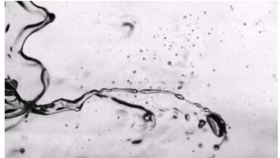
Unstable motion of retracting sheet generates small droplets  $d \leq 50 \mu\text{m}$
