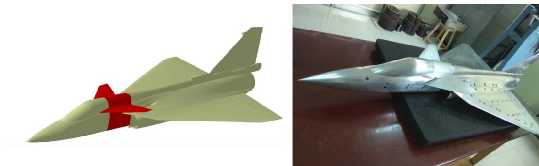
Figure 2: DELTA+PLUG+CANARD configuration used in Wind tunnel tests (shown without missiles).
