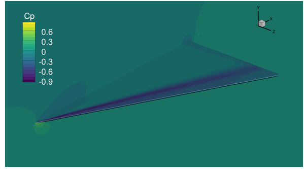
(b) Pressure contours at Mach 0.083, \alpha = 5^\circ
