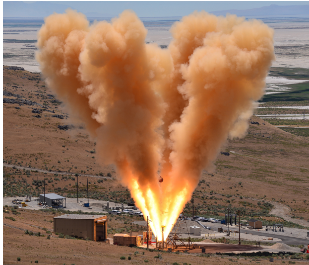
Figure 5: Picture of the Abort Motor Qualification ground test (QM-1) showing the abort motor plumes, the test stand, the PIAT tower (used to measure the IOP wave strength) to the left of the test stand, the two near-field pressure array (NFPA) measurement towers to the right of the test stand, the heat shield measurement apparatus just above the test stand and the crane from which it is suspended further above.
