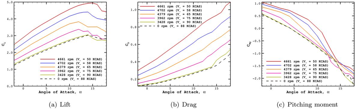
Figure 14: Sample integrated quantities for powered simulations at the 30° flap setting for 10° angle of attack.
