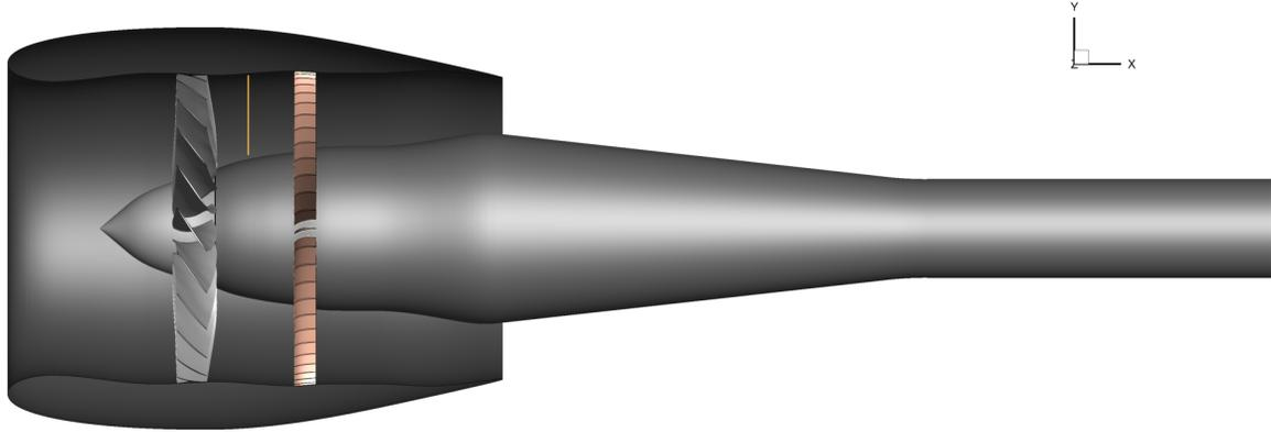
Figure 16: Overview of the SDT geometry with the R4 rotor and baseline outlet-guide-vane (OGV) stages. The light gray surfaces in the centerbody nose (spinner) and rotor represent the rotating components. This rotation is counter-clockwise looking in the +X direction. The yellow line represents the location where single-point hot-wire probe measurements were taken to characterize the rotor wake flow field [58].
