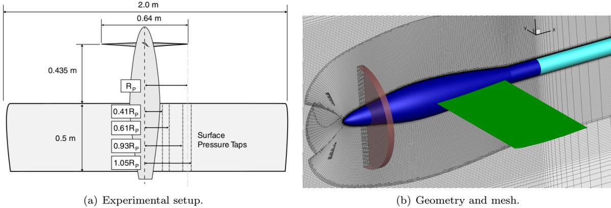
Figure 8: Depiction of experimental setup from Samuelsson [13] (a) and mesh used (b). Area of actuator disk/volume highlighted in red, hub/fuselage with sting extension in blue and wing in green.
