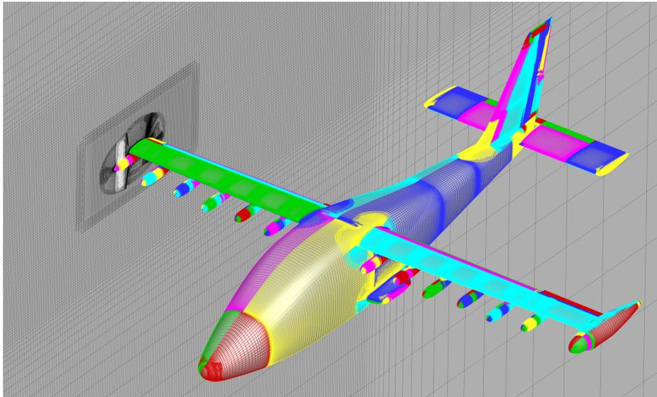
Figure 12: X-57 grid system used for simulating the  $30^\circ$  flap deflection setting with all other control surfaces neutral. Volumetric slice emphasizes an actuator zone shown in white with surrounding body-fitted and off-body domains shown in grey.
