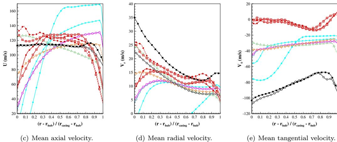
(c) Mean axial velocity. (d) Mean radial velocity. (e) Mean tangential velocity.
