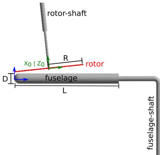
Figure 6: Georgia Tech Rotor-Airframe Model setup [42]
