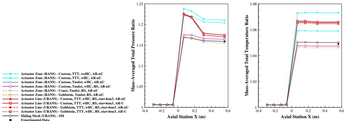
(a) Mass-averaged total pressure ratio along axial stations. (b) Mass-averaged total temperature ratio along axial stations.
