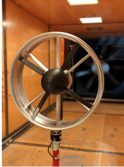
Figure 8: Ducted fan tested in the wind tunnel.
