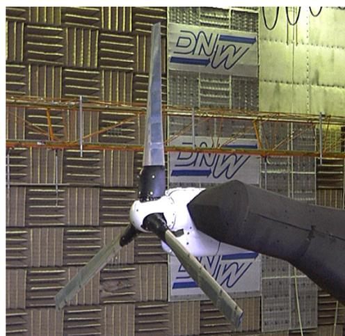
**Figure 3** TRAM 1/4-scale model in airplane mode at the DNW wind tunnel.
