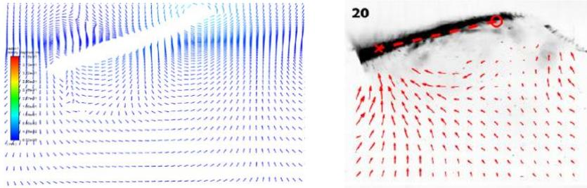
Figure 1: Velocity Plot results from (a) ANSYS Fluent and (b) experiments[1]
