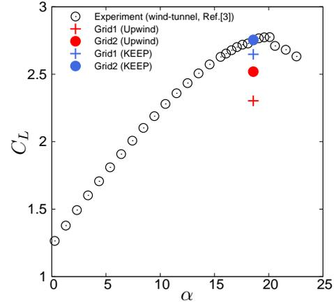
Figure 5: Lift coefficient  $C_L$ .
