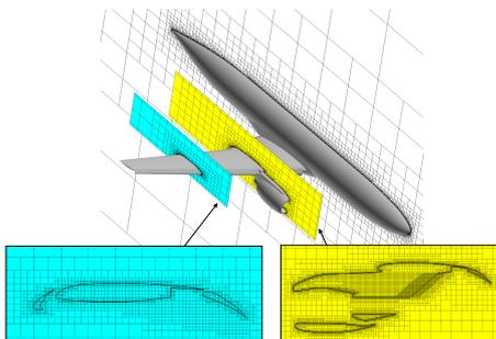
Figure 1: Hierarchical Cartesian grid around JSM.
