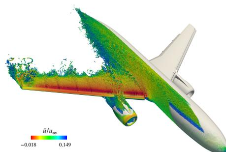
Figure 2: Iso-surfaces of Q criterion.
