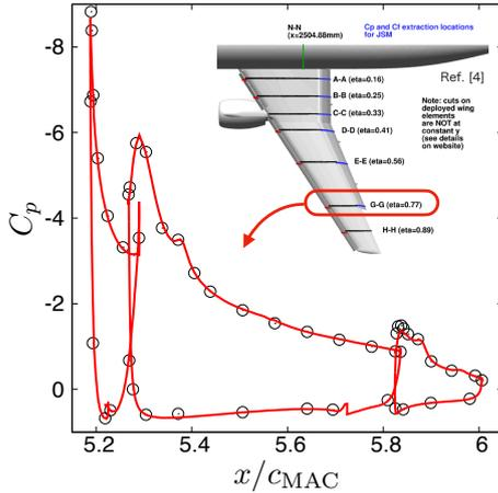
Figure 4: Time-averaged pressure coefficient  $C_p$
