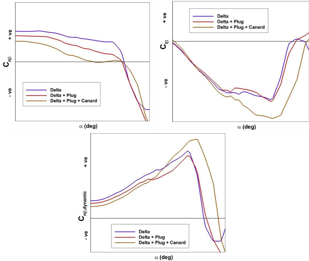
Figure 9: Lateral directional characteristics from Wind tunnel tests.
