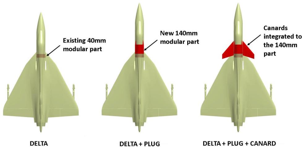
Figure 1: Three configurations tested in Wind tunnel (1:10 scale).
