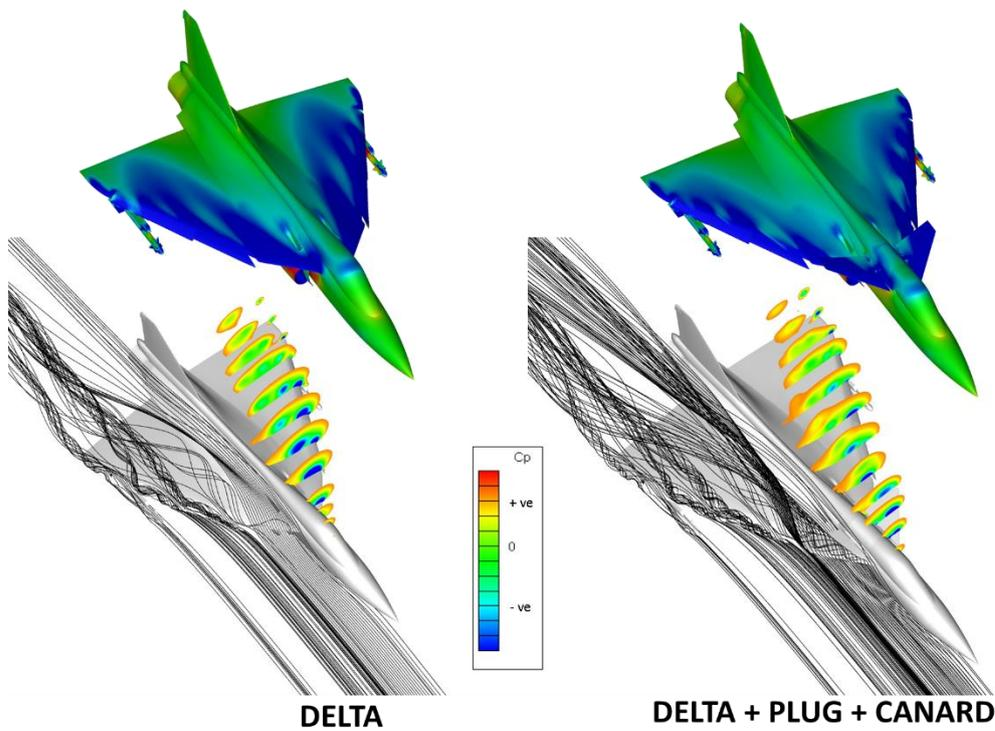
Figure 8: Surface pressure contours from CFD for DELTA and DELTA+PLUG+CANARD for AOA=18°.
