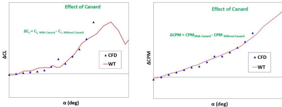
Figure 5: CFD and Wind tunnel results of the delta effect of canard.
