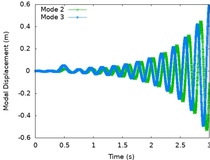
Figure 4. Modal Displacements of Modes 2 and 3 for the  $Q = 60$  kPa Run
