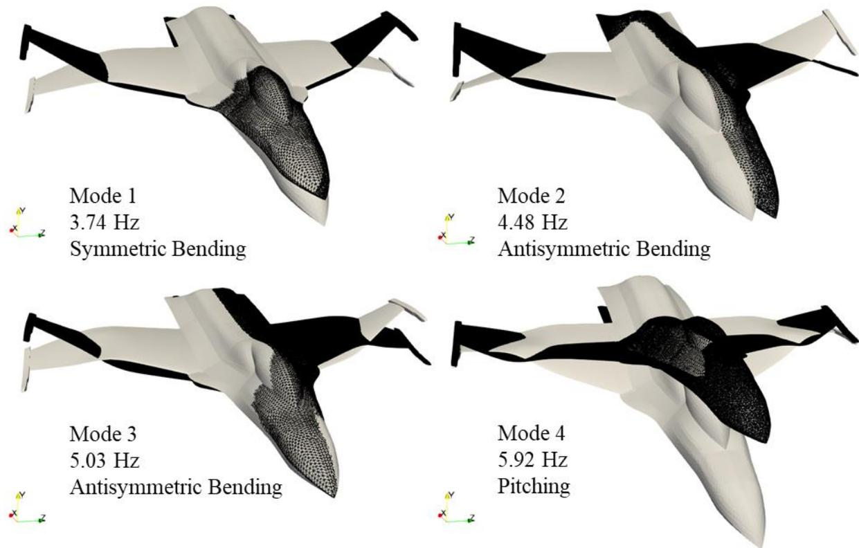
Figure 2. Structural Mode Shapes of the First Four Modes of the Open Source Fighter
