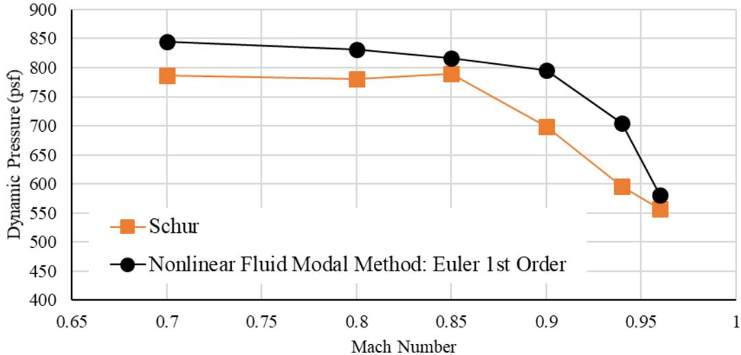
Figure 7. Flutter Boundary for the Open-Source Fighter with Comparisons between the Schur and Nonlinear Fluid Modal Methods
