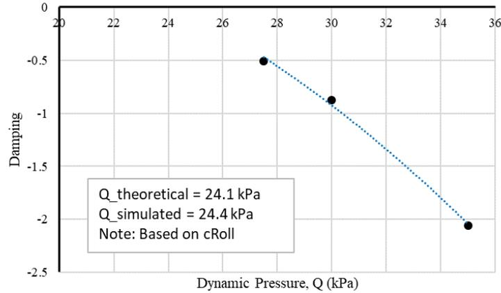
Figure 5. Extrapolation of the Simulated Critical  $Q$  Value of the Open Source Fighter at  $Mach = 0.96$
