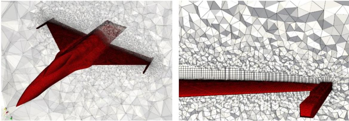
*Figure 1. CFD mesh of the Open Source Fighter*
