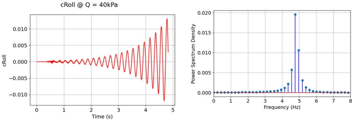
Figure 6. FFT of the Coefficient of Roll of the  $Q = 40$  kPa Simulation Run
