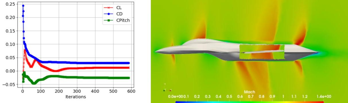
Figure 3. Steady-State Flow Field and Convergence Properties of the  $Q = 60 \text{ kPa}$  Run
