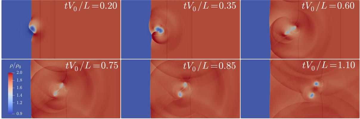
Figure 2: LSV simulation of an inviscid strong shock-strong vortex interaction performed with  $N = 7$  polynomial order in both directions and  $K_x \times K_y = [256 \times 128]$  cells. Six different time instants are shown to illustrate the system's development.
