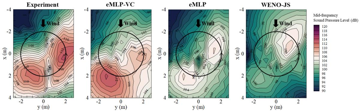
Figure 2. Noise map comparison (HART II, Mid-frequency SPL).
