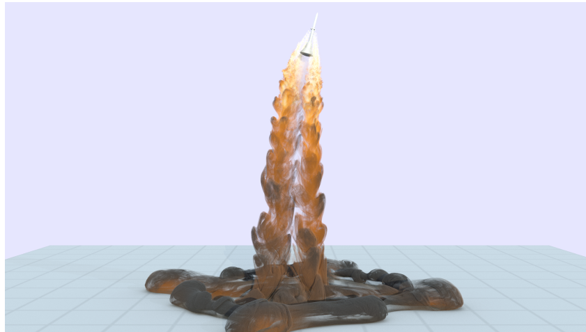
Figure 2: Snapshot from PA1 simulation showing passive particles colored by velocity magnitude (white is high, dark orange is low) seeded at the nozzle exit. A blue tile pattern is used to indicate the position of the ground.
