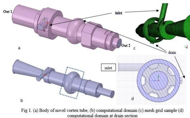
Fig 1. (a) Body of novel vortex tube, (b) computational domain (c) mesh grid sample (d) computational domain at drain section
