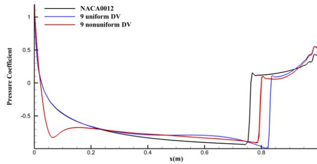
b) Pressure distributions for optimum airfoil shapes
