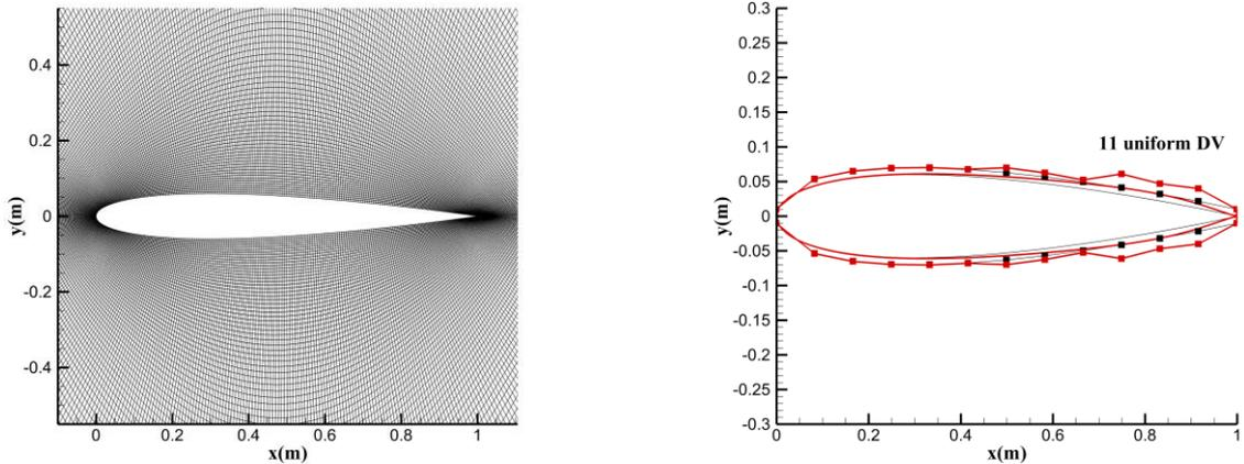
Figure 1: Close-up view of the  $513 \times 257$  O-mesh (left) and stretched Bèzier surface control lattice in red line corresponding to 11 uniform design variables (right).
