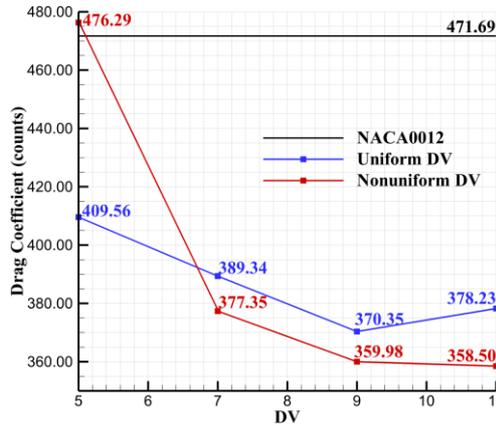
Figure 6: Results for the inviscid optimization of NACA0012 with increased number of variables.
