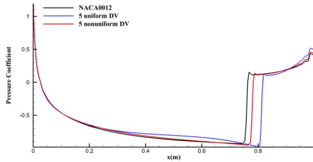
b) Pressure distributions for optimum airfoil shapes
