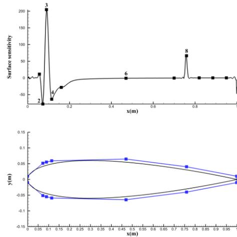
Figure 5: Customized control lattice of 5 design variables determined based on surface sensitivities.
