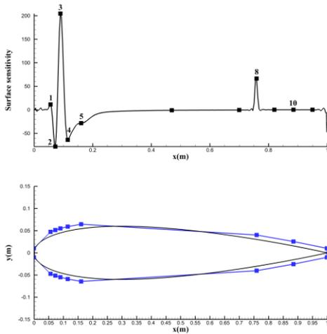
Figure 4: Customized control lattice of 7 design variables determined based on surface sensitivities.
