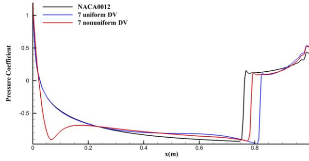
b) Pressure distributions for optimum airfoil shapes
