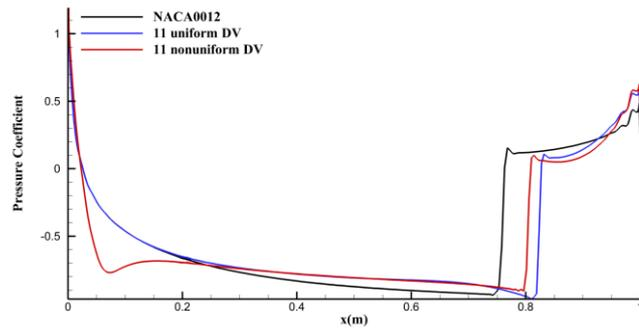
b) Pressure distributions for optimum airfoil shapes
