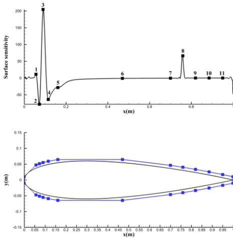
Figure 2: Customized control lattice of 11 design variables determined based on surface sensitivities.
