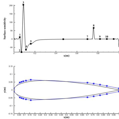
Figure 3: Customized control lattice of 9 design variables determined based on surface sensitivities.
