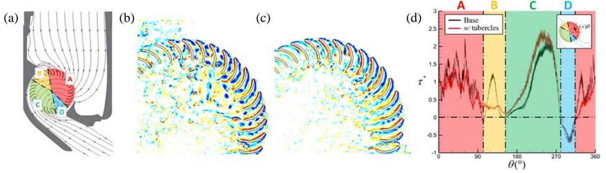
Figure 3: flow characteristics and torque coefficient with and without protrusion: (a) phase averaged streamlines; (b and c) contours of the spanwise vorticity without and with protrusion, respectively; (d) torque coefficient along the azimuthal direction;
