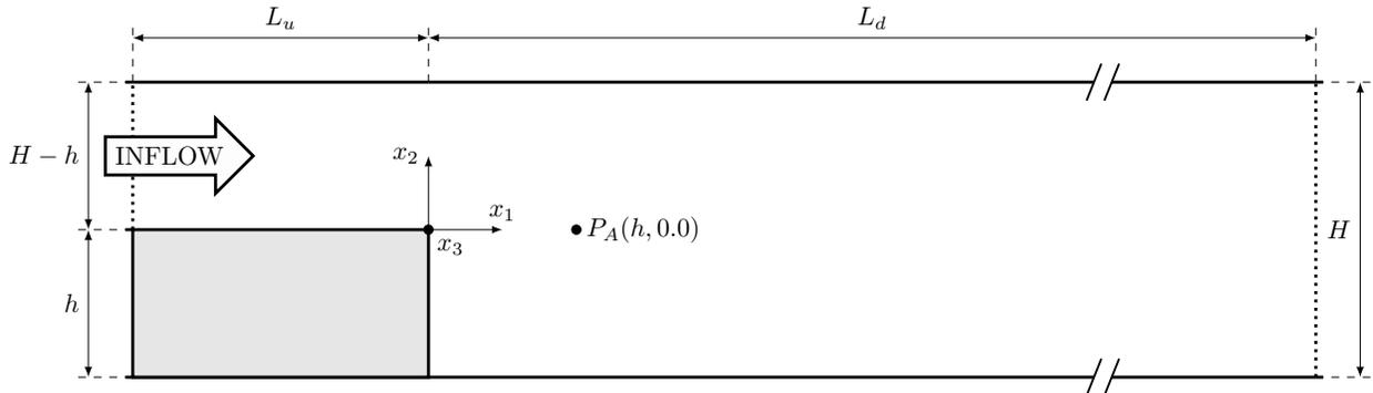
Figure 1: Schematic figure of the Backward Facing Step problem,  $ER = H/(H - h) = 2$ , and details about its geometry and grid spacing (size of zones and concentration factors; arrows indicate the grid refinement direction). Not to scale.
