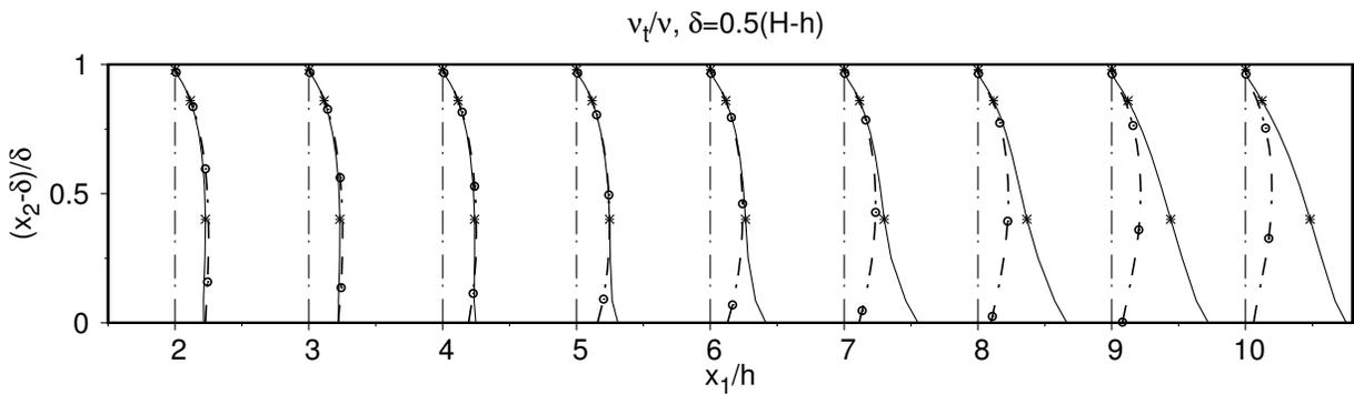
Figure 4: Comparison of the kinematic eddy viscosity vs the kinematic natural viscosity ratio,  $\nu_t/\nu$ , of the DDES-SA. Where DDES-SA data is referred by dashed-dotted lines (- o - ·) and RANS-SA is denoted as (\*—).
