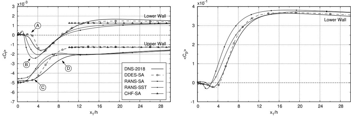
Figure 5: Comparison of the skin friction (left),  $\langle C_f \rangle$ , and the pressure coefficient (right),  $\langle C_p \rangle$  at  $Re_\tau = 395$  of the DNS data with the DDES-SA, the RANS-SA and the RANS-SST results. The  $\langle C_f \rangle$  of a channel flow with the BFS outflow geometry is also displayed (CHF-SA ).
