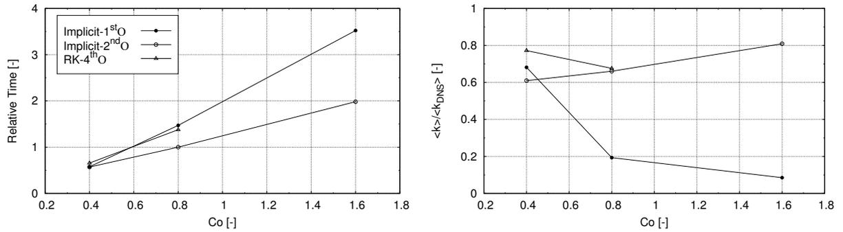
Figure 6: The computational cost (left) of different time integration schemes, including their time step sensitivity,  $Co$ . The turbulent kinetic energy (right) at the point  $P_A$  (Fig.1) resolved by the *coarse-DNS* respect to the the DNS  $\langle k_{DNS} \rangle$ . The computational cost is relative to the *Implicit 2<sup>nd</sup>*-order and  $Co = 0.8$ , which is set to 1.
