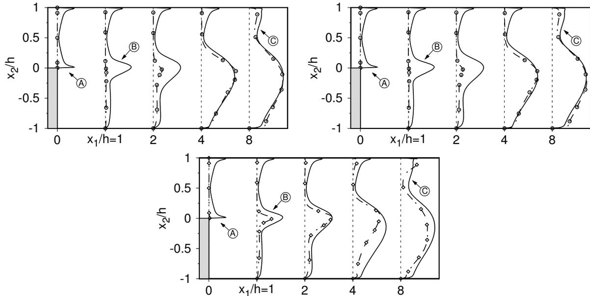
Figure 7: Resolved Reynolds stresses in the stream-wise direction ( $\langle u'_1 u'_1 \rangle$ ) along the recirculation region, using an *Implicit* 2<sup>nd</sup>-order (left) and a *RK* 4<sup>th</sup>-order (right,bottom) with  $Co \sim 0.8$ . Where DDES results (top) are indicated by dashed-dotted-circled lines (- o - ·) and the *coarse-DNS* (bottom) data is referred by dashed-dotted lines (- ◊ - ·). DNS results are represented by solid lines (—) in both graphs.
