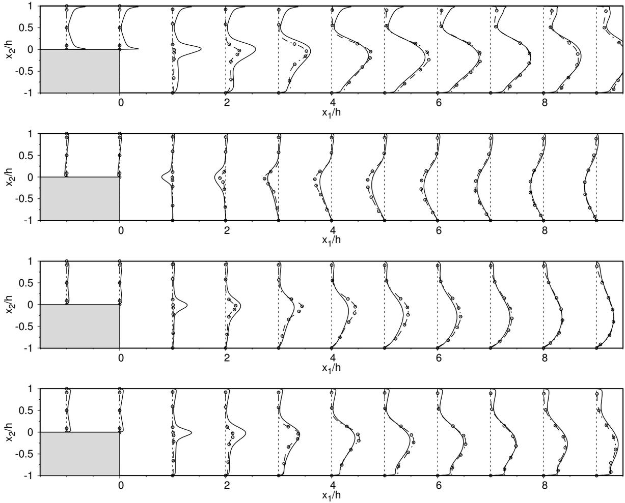
Figure 3: Resolved Reynolds stresses in the stream-wise ( $\langle u_1' u_1' \rangle$ , top), crossed ( $\langle u_1' u_2' \rangle$ , middle-top), normal ( $\langle u_2' u_2' \rangle$ , middle-bottom) and spanwise ( $\langle u_3' u_3' \rangle$ , bottom) directions along the recirculation region. Where DNS results are indicated by solid lines (—) and the DDES-SA data is referred by dashed-dotted lines (- o - ·).
