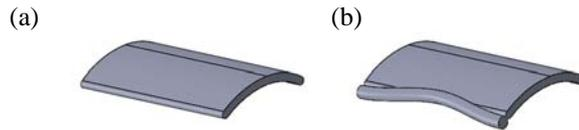
Figure 2: (a) Base blade; (b) blade with a sinusoidal protrusion on the leading edge of each blade.
