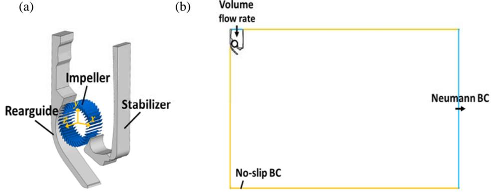
Figure 1: (a) Schematic diagram of a cross-flow fan; (b) computational domain and boundary conditions.
