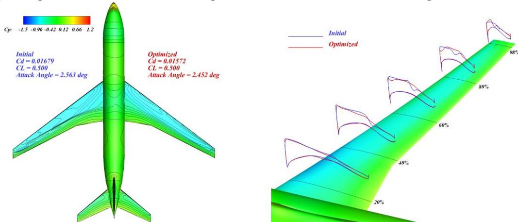
Figure 6: Comparison of the optimization results with the baseline configuration.
