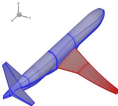
Figure 1: Mesh generation for CRM Wing-Body-Tail
