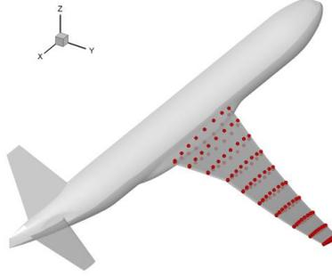
Figure 2: The shape design variables are the z-displacements of 160 FFD control points
