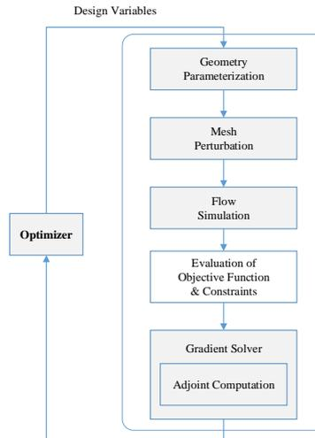
Figure 4: The main framework for aerodynamic shape optimization
