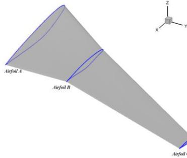
Figure 3: The constrained airfoil sections
