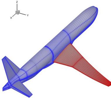
Figure 1: Mesh generation for CRM Wing-Body-Tail
