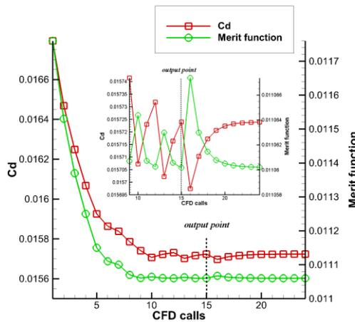
Figure 10: Number of objective evaluation vs. the merit function value and the drag coefficient.
